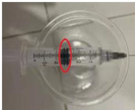
Figure 6. Volume of nutrient solution delivered by the peristaltic pump after 1 minute of operation.
